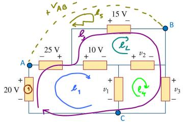
1. Use KVL to obtain  $v_1$ ,  $v_2$ , and  $v_3$ .
